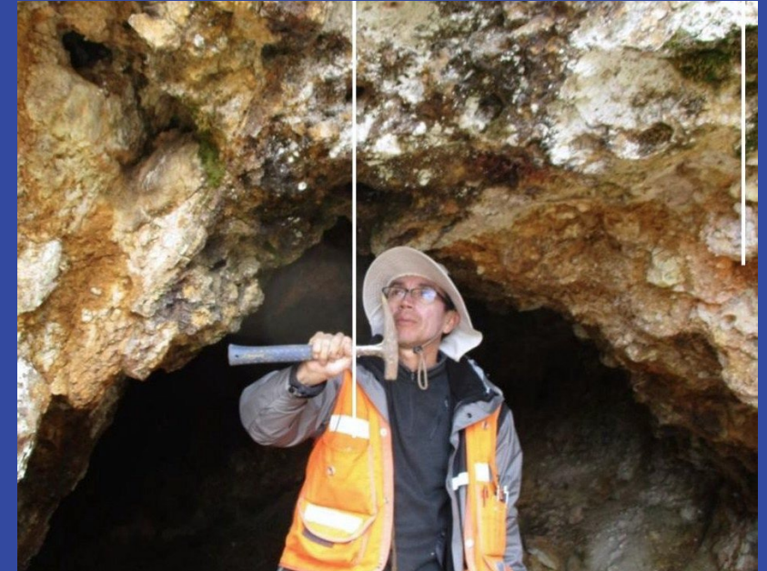
Vein facing east-southeast, showing clayey-looking Huancané conglomerates forming walls to darker, well defined mineralized structure.
